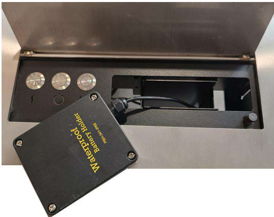
Fig. 9 – Removing of the battery container
