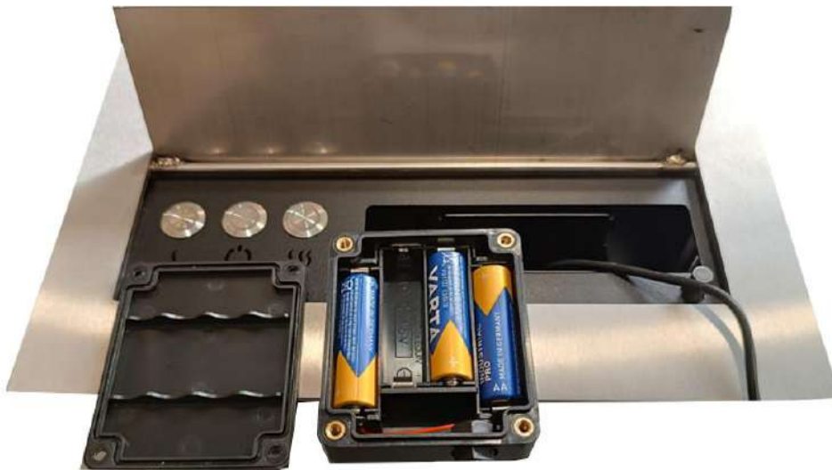
Fig. 11 – Putting back the battery box
