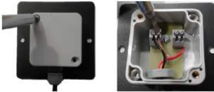
Fig. 12 – Closing the back of the wallswitch
