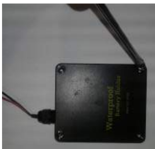
Fig. 20 – Unscrewing battery box
