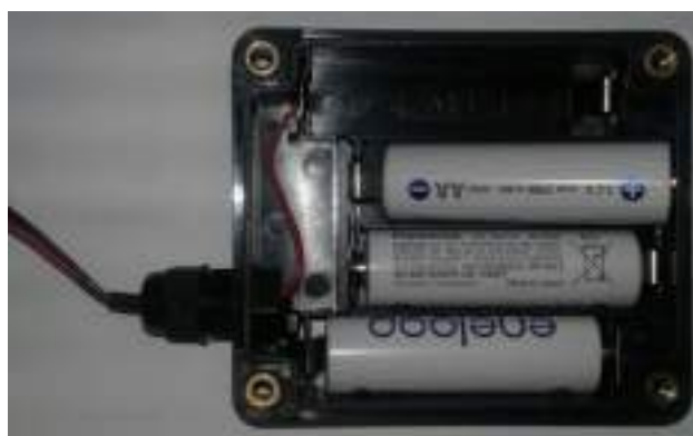
Fig. 21 – Replacing battery in battery box
