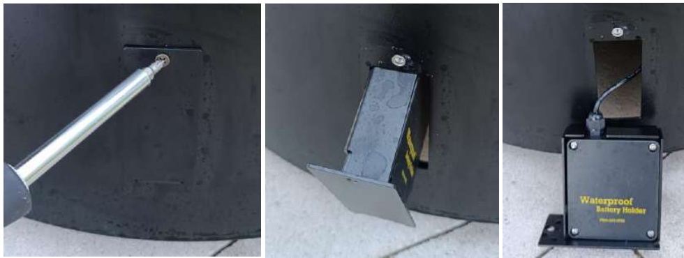
Fig. 8: Removing of the battery container
