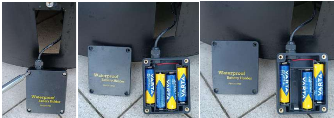
Fig. 9: Replacing the batteries in the container
