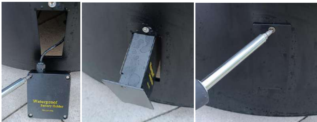
Fig. 9: Replacing the batteries in the container
